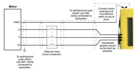
Figure 7 - Motor connections
